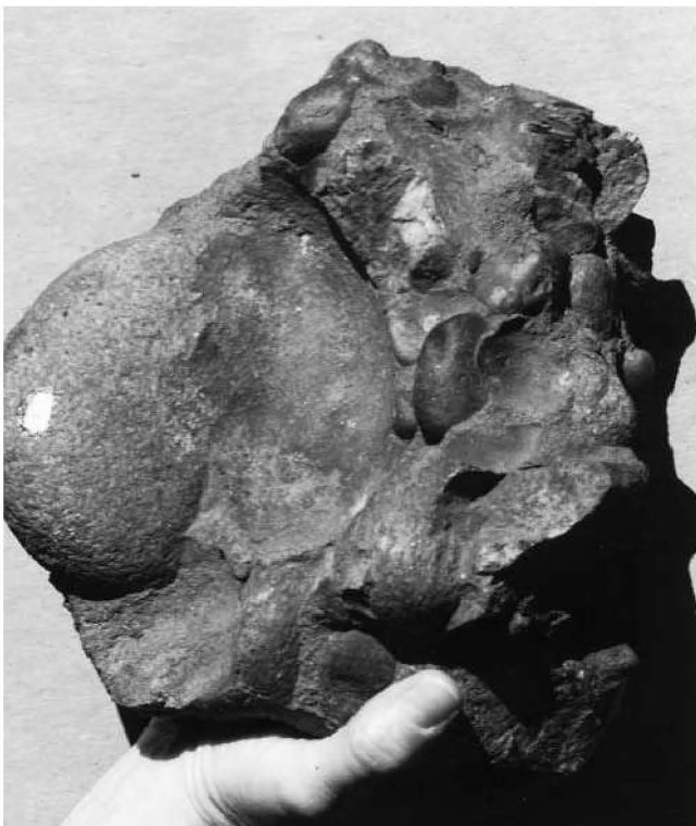
FIGURE 1.1 Hand sample of a coarse, poorly sorted conglomerate with well-rounded cobble- and pebble-sized clasts. (Photo by D. R. Prothero.)
